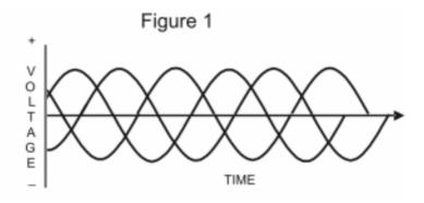
This consists of 3 separate phase conductors along with a neutral conductor transmitting supplies to a given destination.
