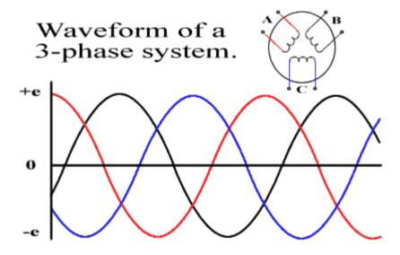
Such an arrangement would provide us with a 3 phase supply but we would need 6 conductors in order for it to function. However if we take each coil and interconnect it with the other coils in particular ways we can achieve a three phase supply in either a 3 wire (Delta) system, or a 4 wire (Star) system.
