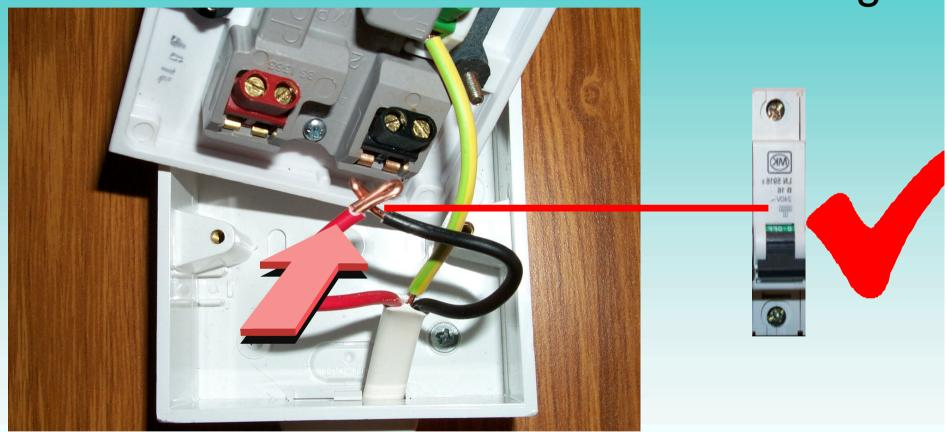
Large fault current flows - fuse or circuit breaker should operate
