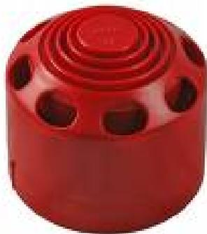
Normally red and alerts occupants audibly to a fire. These can be supplemented by visual alarms ( flashing beacons ) where areas can be normally noisy i.e. factories or DDA compliance. General sound level required is 65 DBa or 75 DBa in a room of sleep at bed head level. The sounder can also be integrated with a smoke or heat detector making it an ideal option for bedrooms where the owner might not want to see a red sounder on the wall.
