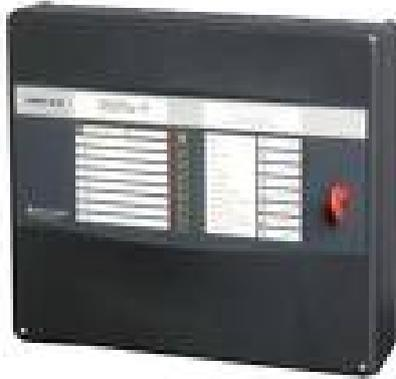
The basic technology is Non-Addressable which is found more often in smaller buildings due to it being more cost effective. A non-addressable system is simply comprised of Fire zones. These are represented by red l.e.d.s on the control panel. Faults use amber l.e.d.s.
