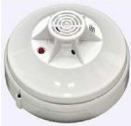
Comes in two variants and are most commonly found in kitchens, boiler rooms or unclean environments. They come as Rate of Rise which detects a rapid increase in temperature or fixed temperature which will only activate after the room temperature exceeds a pre determined temperature set into the detector.
